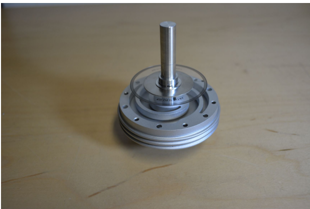
Fig. 4. A series elastic unit consisting of output spring shaft, elastic element, and input pulley (below the spring). The output pulley contains its own shaft that is integrated into the custom pulley. The spring has an integrated hub for connection to its own output shaft. These monolithic concepts reduce a possible point of failure between the connection of the spring and pulley to their respective shafts.
